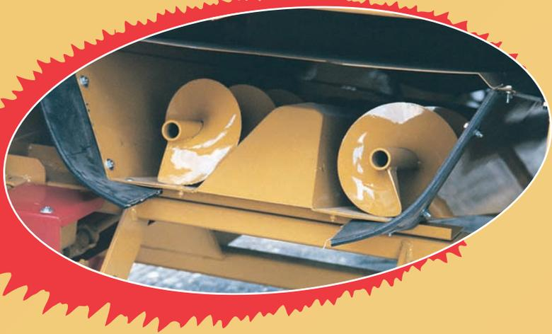
The two heavy-duty and high capacity augers mounted in the **belly pan**, convey the product to the discharge conveyor. The auger and pan combination provides for a high-speed transfer of the product and for a clean, leak-free environment under the tub grinder.
